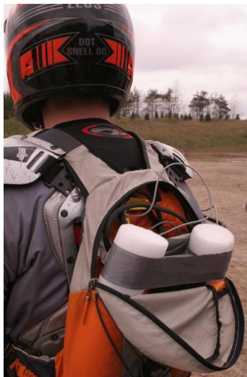
Portable VO<sub>2</sub> testing computer
